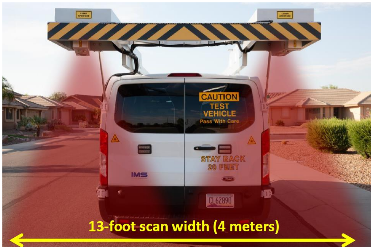
Figure 6 – RST Equipped with the 3D LCMS-2 Camera
