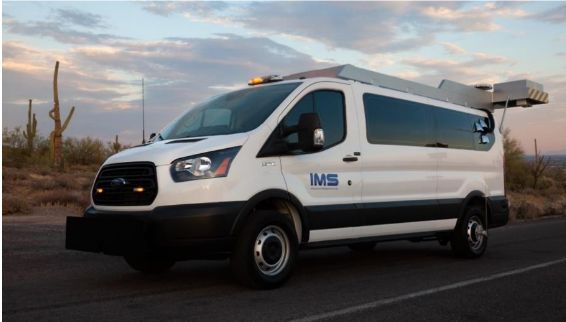
Figure 5 – Laser Road Surface Tester (RST)
