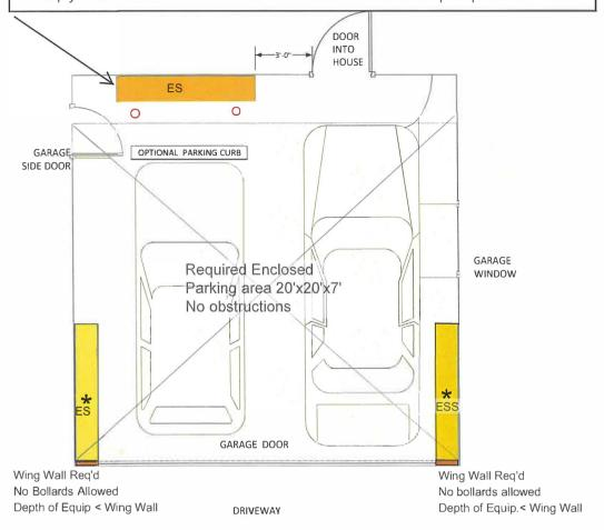
→ Allowable areas for Wall Mounted ESS. 96" from garage entry &12" Max. Projection from Wall Do not block front door swings for drive or front passenger
