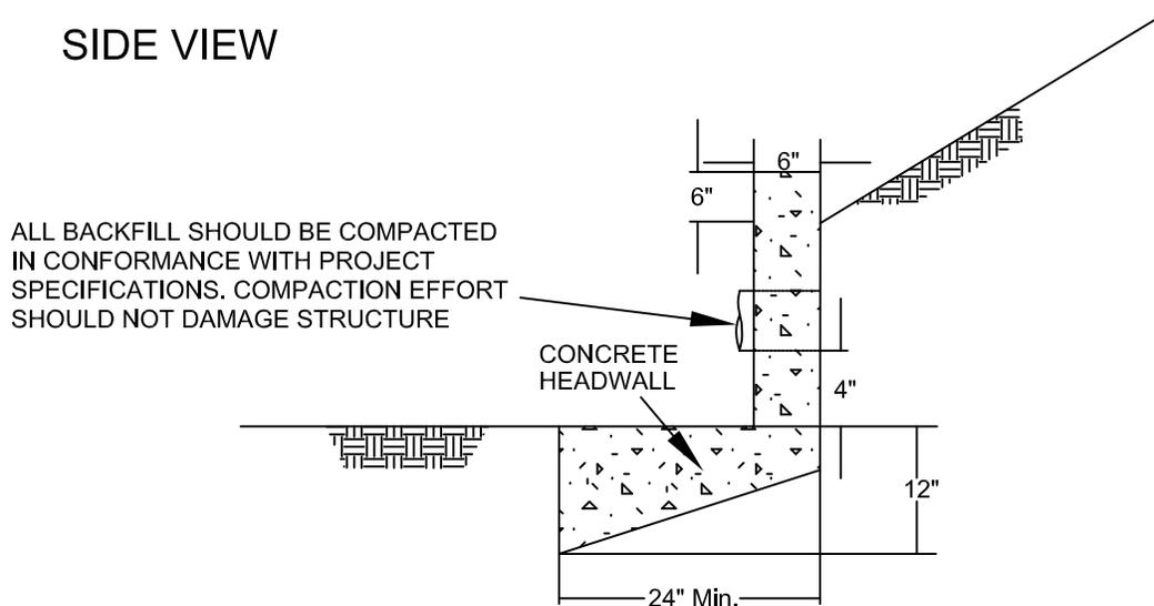
NOTE: HEADWALL SHOULD OUTLET AT TOE OF SLOPE
